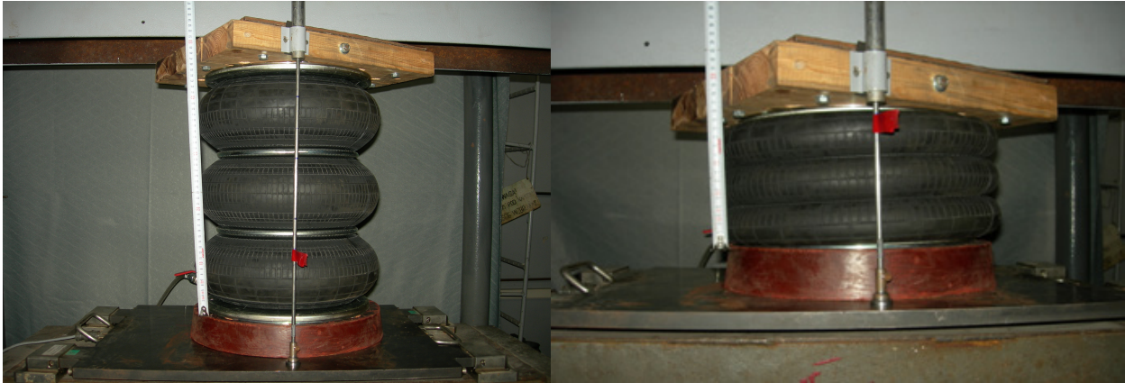
Fig. 4. Tests of the pneumatic shock absorber (pneumatic bellows): a) location of the maximum operating length, b) location of the minimum operating length
