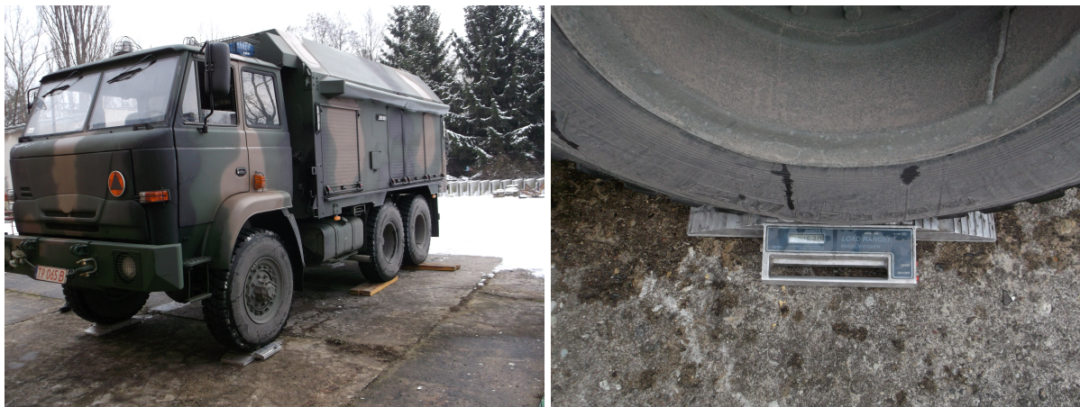
Fig. 2. Weight distribution testing for STAR 266M2 vehicle with special body
