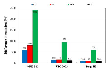
Fig. 2. Relative difference in emissions of harmful substances (Stage IV = 100%)
