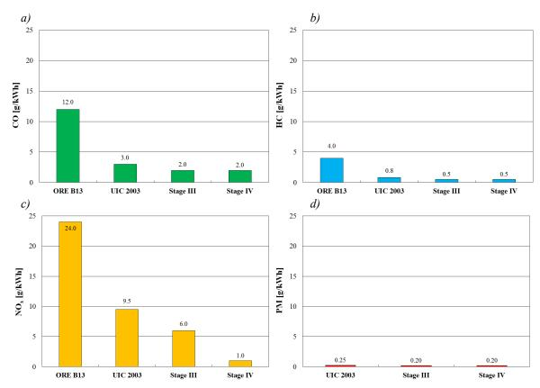
*Fig. 1. The emission values of the individual toxic compounds for the respective emission standards of locomotives [10]: a) carbon monoxide, b) hydrocarbons, c) nitrogen oxides, d) particulate matter*
