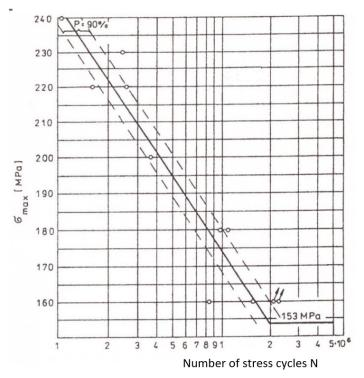
Fig. 5. Wöhler diagram for welded joints of quenched sheets 12 mm thick of S640Q steel with R = -0.3
