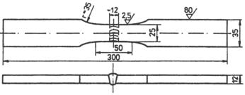
Fig. 4. Samples used for fatigue tests with weld nobs left in place
