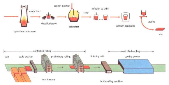
Fig. 2. Diagram of TMCP steel production line used by Nippon Steel Corporation [1, 7]
