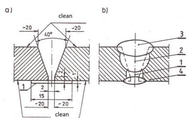
*Fig. 3. The scheme of welding: a) sheets edges preparation: 1 – copper pad, b) welding sequence: 1 – before penetration run, 2 – filling run, 3 – closing run*
