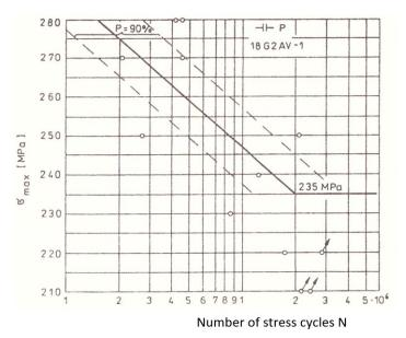
Fig. 6. Wöhler diagram for welded joints of quenched sheets 12 mm thick of S640Q steel where R = 0.3 and welds edges were penetrated by TIG method without adding filler metal
