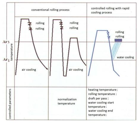
Fig. 1. Comparison of rolling processes [7]
