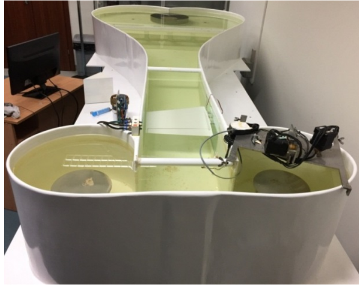
Fig. 5. Wing model prepared for the visualization test inside the water tunnel
