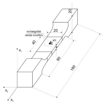
Fig. 1. Geometry of the sample, dimensions and anatomical directions  $x_1$  – radial direction,  $x_2$  – tangent direction,  $x_3$  – longitudinal direction
