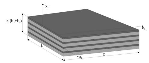
*Fig. 2.* The geometry of the measuring part of the sample (see Fig. 1): *c* – length of the measuring part, *b* – measurement part width, *k* – measurement part thickness
