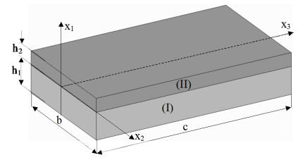
Fig. 3. Sample measuring part oriented in a rectangular coordinate system: I – soft layer, II – hard layer
