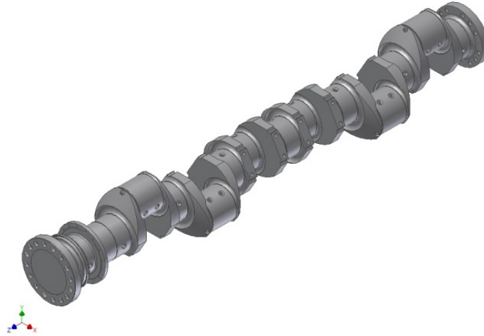
Fig. 1. The 3D model of the monolithic marine diesel engine crankshafts type 12V38
