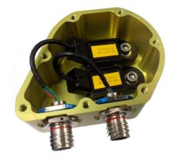
Fig. 5. Air pressure sensors in custom-made protective casing
