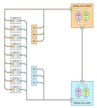
Fig. 3. Setup of control units of the ignition system
