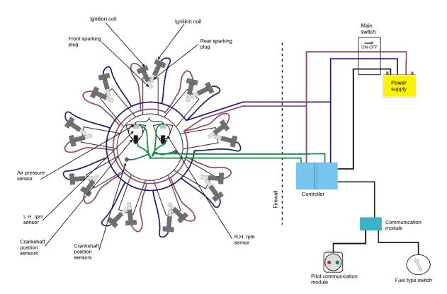
Fig. 2. Electronic ignition system
