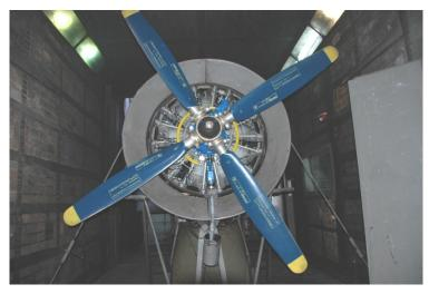
Fig. 1. ASz-62IR-16E Engine on test stand. Front view
