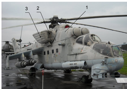
Fig. 7. Mi-24 Hind helicopter after modernization, 1 – engine, 2 – exhaust cooler air intake, 3 – exhaust cooler [6]
