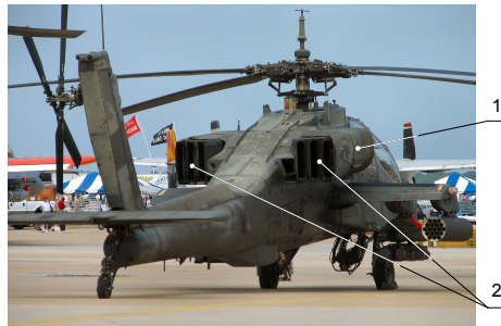
Fig. 6. AH-64 Apache rear view, 1 – engine, 2 – exhaust cooler [14]
