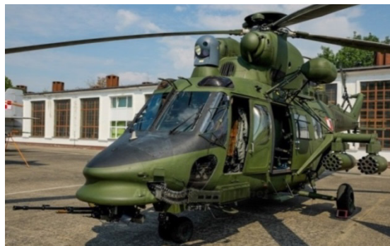
Fig. 9. Helicopter in combat support version W-3PL Gluzec [6]
