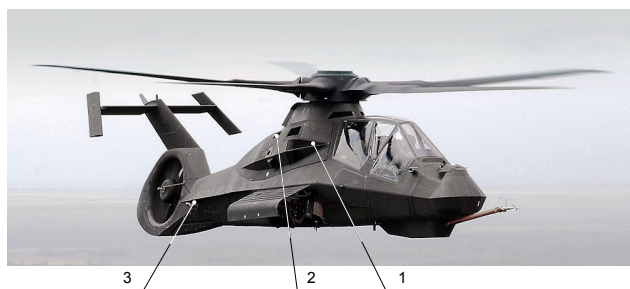
Fig. 8. RAH-66 Comanche prototype in flight: 1 – engine air intake, 2 – exhaust cooler air intake, 3 – exhaust system [6]
