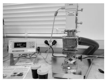
Fig. 1. The Vibro Viscometer SV 10
