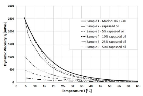
Fig. 2. Graph of viscosity-temperature changes for all samples
