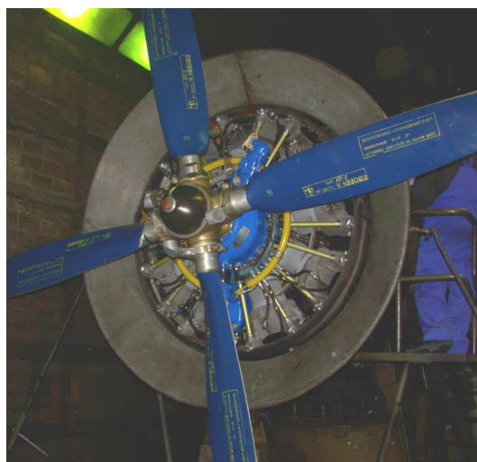
Fig. 1. ASz-62IR-16E engine in test bed
