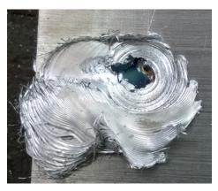
Fig. 7. View of broken FSW tool into 5083 alloy sheet - result of joining with too low temperature
