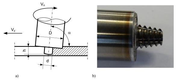
Fig. 1. The diagram of FSW (a) and view of tool used in research (b)
