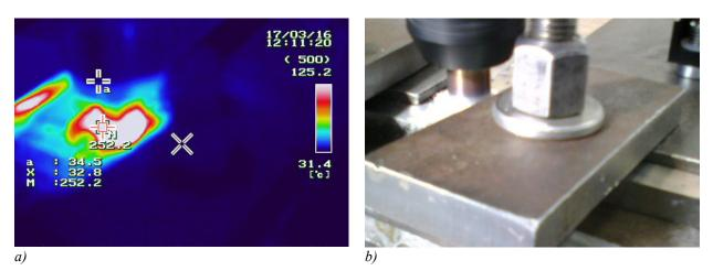
*Fig. 4. Thermogram (a) and visual picture (b) of FSW process during plasticizing – medium temperature in contact point (252.2°C)*
