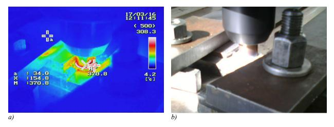
*Fig. 5. Thermogram (a) and visual picture (b) of FSW process during plasticizing – sufficient temperature to start welding (370.8°C)*
