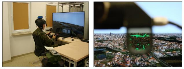
Fig. 4. Demonstration Station for new functions testing of Helmet-Mounted Display Systems [11]
