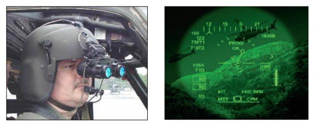
Fig. 1. The ANVIS Helmet-Mounted Display System for AH-1 military helicopters [8]
