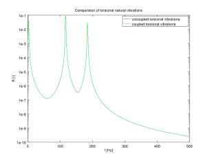
Fig. 6. The spectrum of natural displacements of torsional vibrations of the model of the crankshaft with the coupling
