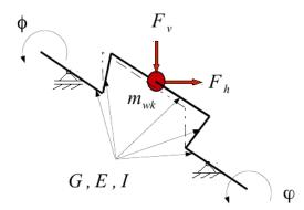
Fig. 1. The model of the crankshaft of the one piston
