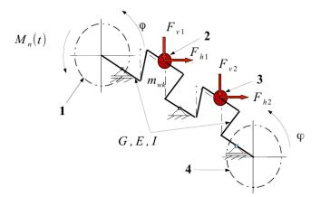
Fig. 2. The model of the crankshaft with two pistons
