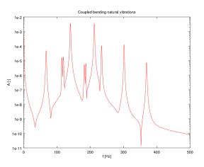
Fig. 1. Bending vibrations of the crankshaft of the system with a coupling
