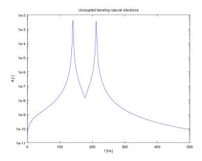
Fig. 5. The spectrum of natural displacements of bending vibrations of the model of the crankshaft without the coupling
