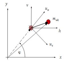
Fig. 3. The model of the single crank of the considered crankshaft
