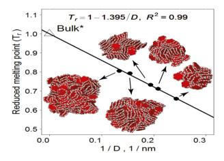
Fig. 4. Relation between reduced melting point and diameter of the clusters of PAH [4]
