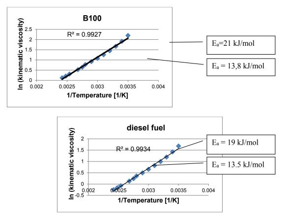
Fig. 2. Activation energy  $E_a$  of disruption reaction of intermolecular bonds, calculated for FAME (B100) and diesel fuel
