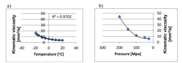
Fig. 3. The mineral diesel fuels viscosity change a) by cooling and b) by increase of the pressure
