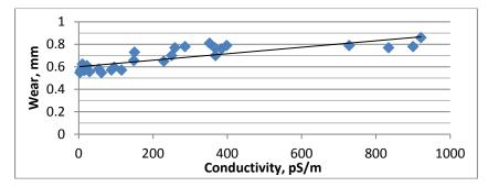
Fig. 7. Relationship between wear after BOCLE test obtained for the number of Jet fuel blends with synthetic hydrocarbons and alcohols and conductivity of these blends
