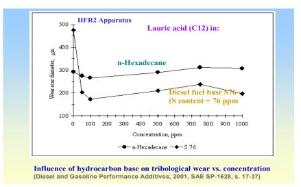
Fig. 6. The relationship between the result of HFRR test (balls wear) and additive (lauric acid) concentration [6]
