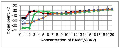
Fig. 5. Cloud point and freezing point change with the increase of FAME concentration in jet fuel; each line represents blend of jet fuel (two kinds of this fuel) and FAME (from two plants) [5]
