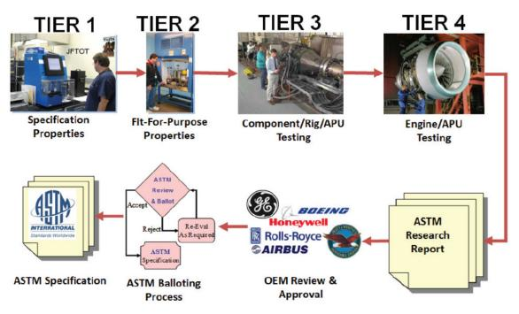
Fig. 3. The algorithm of new synthetic biojet fuels authorization according to ASTM D 4054 standard [8]
