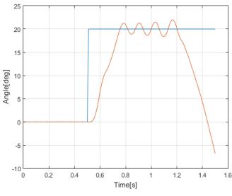
Fig. 6. Step response with large P and D
