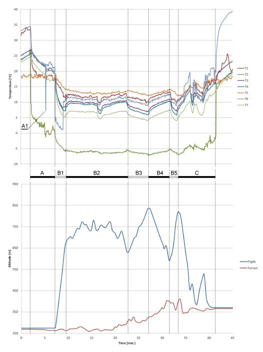
Fig. 2. Visualization of temperature and flight altitude changes in flight from Konopiska to Lgota Murowana on September 24, 2011
