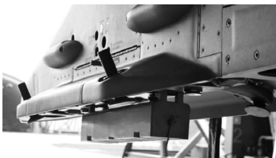
Fig.6. Bomb adaptor suspended on a bomb station of the F-16 aircraft (own photo)
