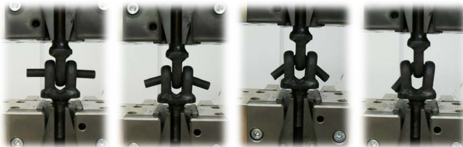
Fig.10. Phases of shearing steel (own photo)
