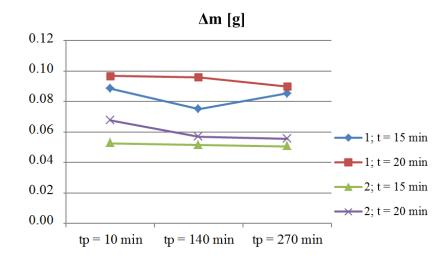
Fig. 6. Dependence between  $\Delta m$  and tp, and t for BC-F400: 1 - v = 27 m/min, p = 0.051 MPa; 2 - v = 38 m/min, p = 0.03 MPa
