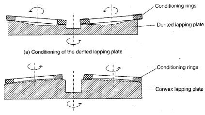
(b) Conditioning of the convex lapping plate Fig. 1. Conditioning methods of the lapping plate with a conditioning rings [9]
