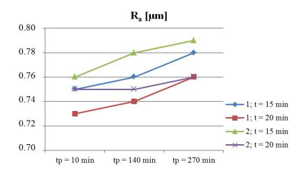
Fig. 7. Dependence between  $R_a$  and tp, and t for BC-F400: 1 - v = 27 m/min, p = 0.051 MPa; 2 - v = 38 m/min, p = 0.03 MPa
