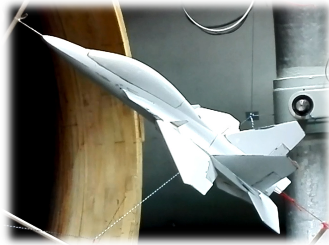
Fig. 9. A quasi-free test of a remote-controlled model in the wind tunnel
