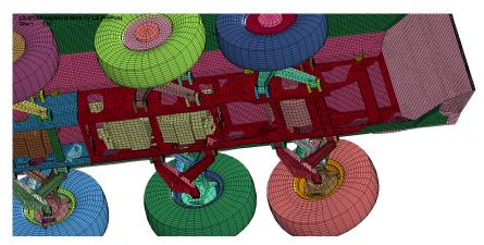
Fig. 6. Deformations of the element of the construction of the underbody (chassis and suspension) resulting from noncontact explosion
