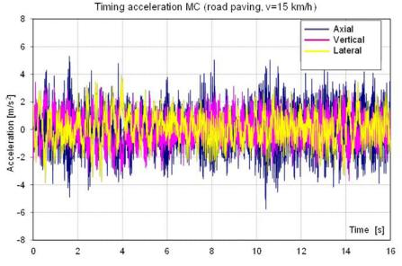
Fig. 2. Accelerations acting on the centre of mass of the tank over time during the travel with v = 15 km/h
