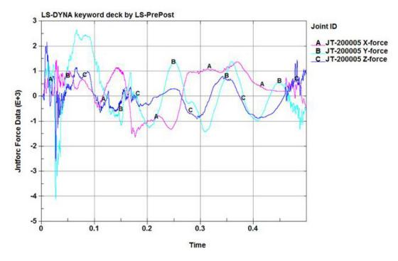
Fig. 9. Change of forces over time at the joint of the load-bearing structure of the anti-aircraft launcher
