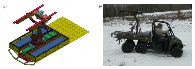
Fig. 8. "Kusza" anti-aircraft weapon system: a) model, b) anti-aircraft launcher on Polaris Ranger 6x6 underbody during training ground tests under winter conditions
