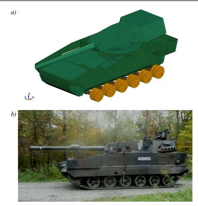
Fig. 1. Light tank: a) model, b) Anders technology demonstrator during a road test
