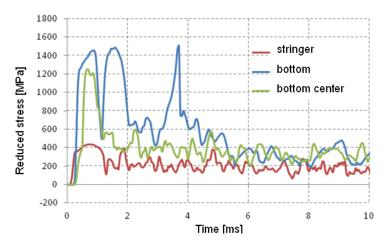
Fig. 4. Changes in tensions in selected structural nodes resulting from non-contact explosion
