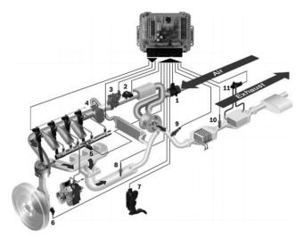
Fig.1. System diagram of diesel engine sensors: 1 – air mass sensor, 2 – boost pressure sensor, 3 – butterfly valve, 4 – exhaust gas recirculation valve, 5 – rail pressure sensor, 6 – speed sensor, 7 – accelerator pedal module, 8 – exhaust temperature sensor, 9 – Lambda sensor, 10 – exhaust temperature sensor, 11 – differential pressure sensor [12]
