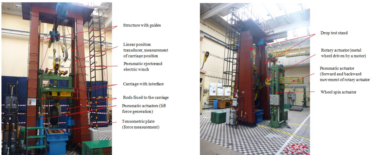
Fig. 2. 10-ton drop test stand
