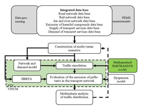
Fig. 2. EMITRANSYS model elements in VISUM
