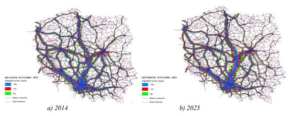
Fig. 7. Exhaust emission of harmful compounds due to the EURO standards a) in 2014 – for the current vehicles structure, b) in 2025 for the change in vehicle structure
