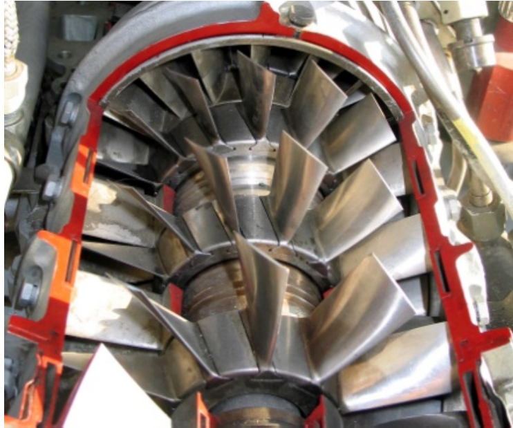
Fig. 1. View of first stages of compressor
