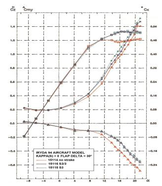
Fig. 2. Aerodynamic characteristics of aircraft model  $Cz(\alpha)$ ,  $Cx(\alpha)$  and  $Cmy(\alpha)$  with and without strake in various variants (slotted flap  $\delta_K = 30^\circ$ ) [6]
