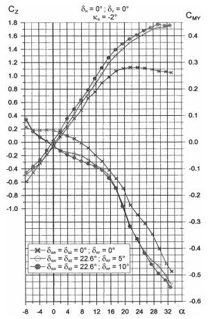
Fig. 4. Aerodynamic characteristics of the aircraft model  $Cx(\alpha)$ ,  $Cz(\alpha)$  and  $Cmy(\alpha)$  with the selected variant of strake with Fowler flap and hidden slot as well flap and slot in a manoeuvring position angled by o  $\delta_{KF} = 5^{\circ}$ and  $\delta_{KF} = 10^{\circ}$  [7]
