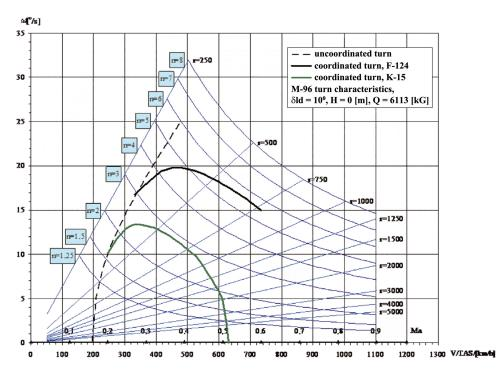
Fig. 9. Characteristics of steady and unsteady turn for aircraft with mounted LERX and the flap in a manoeuvring position with thrust;  $2 \times 1500 \text{ daN}$  and thrust  $2 \times 2833 \text{ daN}$  for height; H = 0 m [4, 10]
