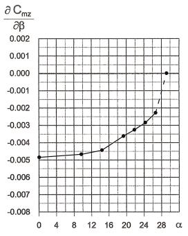
Fig. 5. Dependence of  $\delta Cmz/\delta\beta$  on the wing angle of attack for the tested configurations of the model of aircraft with a band and a swivelled wing flap in the manoeuvring position [7]
