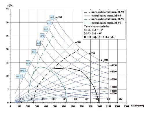
Fig. 8. Characteristics of steady and unsteady turn radius versus speed for I-22 "Iryda" plane before and after its modernization with the flap in a manoeuvring position for height H=0 m [4, 10]
