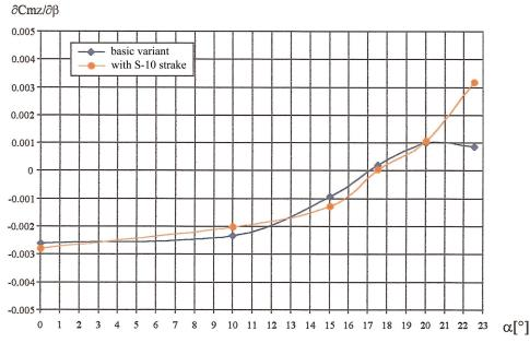
Fig. 3. Relation of  $\delta Cmz/\delta\beta$  in the function of angle of attack of the aircraft model with and without strake [18]
