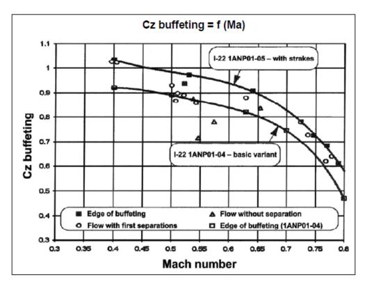
Fig. 7. Comparison of the lift factor at initial buffeting vibrations of aircraft prototype with mounted strake and without mounted strake [5, 12]
