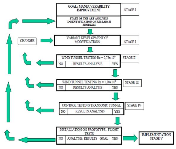
Fig. 1. Design and testing method algorithm [3]
