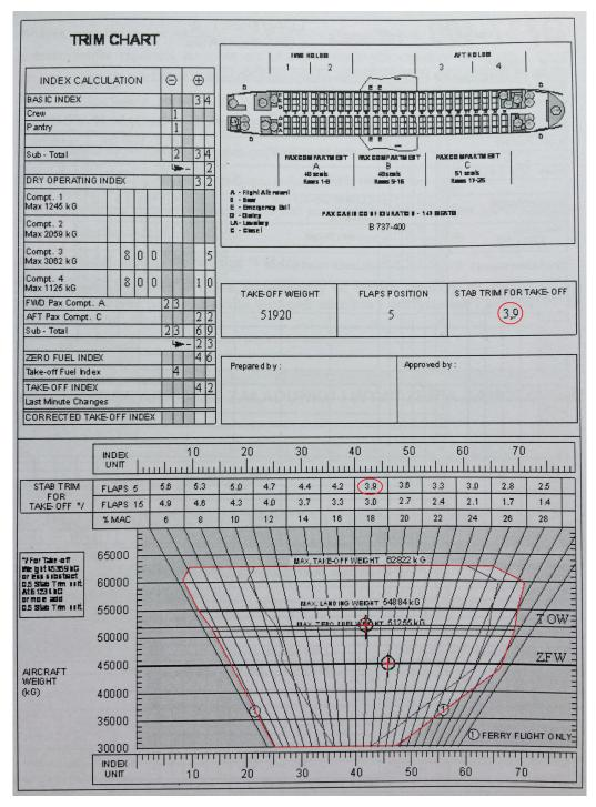
Fig. 7. Example of the completed balance sheet of the Boeing B737-400 aircraft
