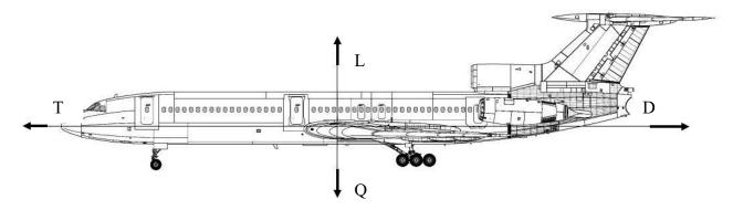
Fig. 1. The distribution of forces on the example of the aircraft
