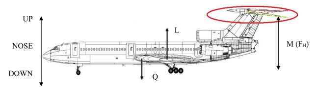
Fig. 3. The principle of operation of the horizontal tail of the aircraft
