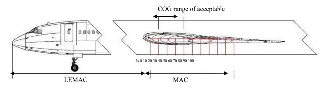
Fig. 5. Graphical representation of the allowable position COG
