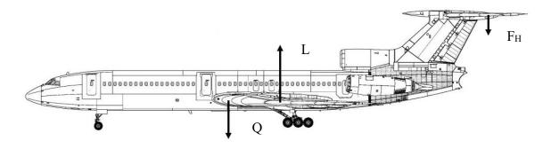
Fig. 2. The distribution of forces on the example of the aircraft
