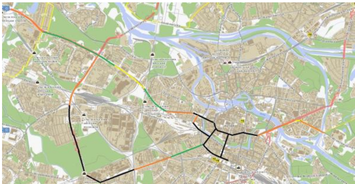
Fig. 3. The route in mobile testing in Wrocław, together with the characteristics of the flow of traffic (in black – the complete road blockage across the width of the road, the car stopped for more than 30 minutes – the average traveling speed in the road section not exceeding 5 km/h; in orange colour – partial blockage of the road, vehicle stoppage for approx. 20-30 minutes – the average traveling speed on the road section up to 10 km/h; in yellow – the road passable, but the movement is gradual; in green – the no road congestion)
