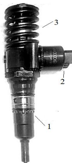
Fig. 2. PDE 2 fuel unit injector subdivided into its components: 1 – nozzle unit, 2 – solenoid section, 3 – fuel-pumping element
