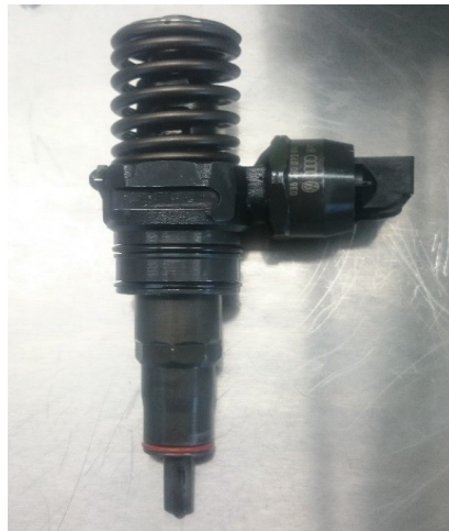
Fig. 10. Fuel unit injector being tested, with a catalogue number 0414720313
