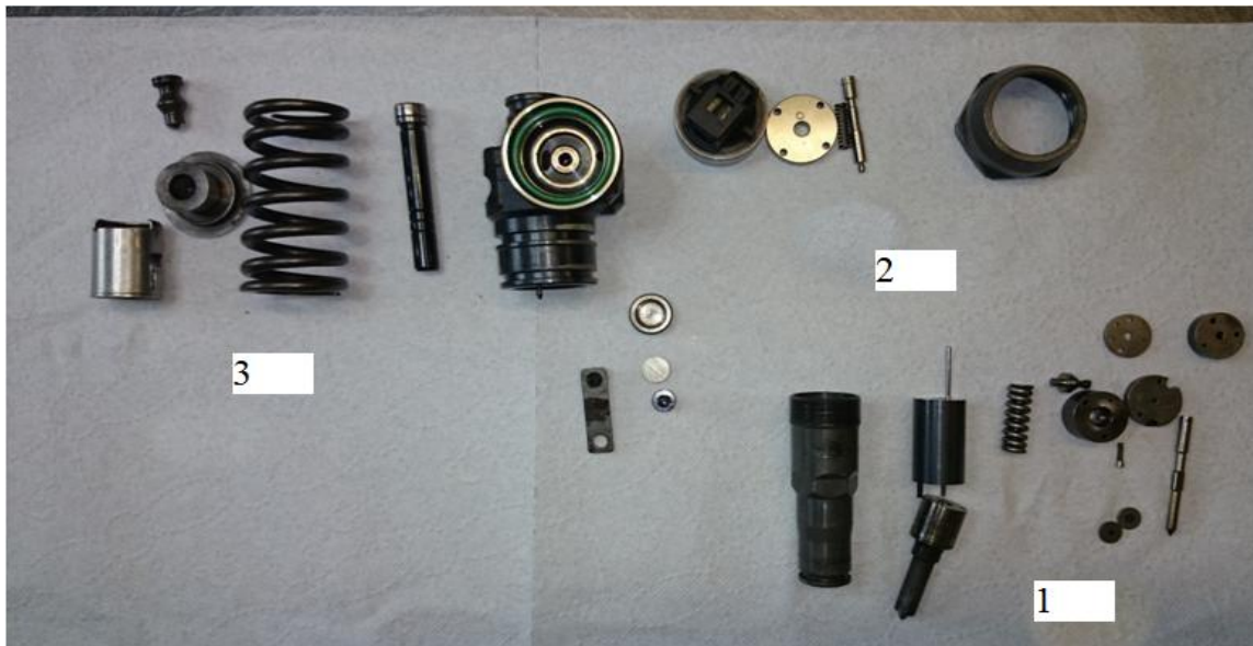
Fig. 3. Disassembled fuel unit injector subdivided into its particular assemblies: 1 – nozzle unit, 2 – solenoid section, 3 – fuel pumping element
