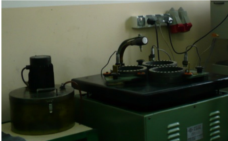
Fig. 3. One-side lapping machine ABRALAP 380
