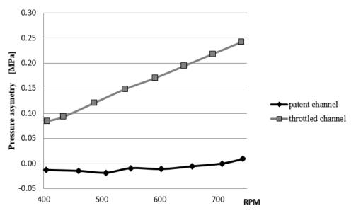
Fig. 5. Effect of channel throttling on compression curve asymmetry
