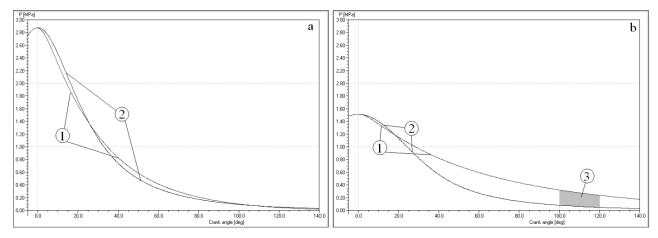
Fig. 4. The measurement of the asymmetry of compression curve with no load at engine speed 700 RPM: a) for the clean channel b) for channel partly chocked: 1) the expansion curve, 2) the mirror image of the compression curve 3) measure of the asymmetry
