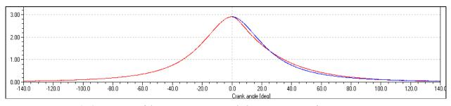
Fig. 2. Comparison of the expansion curve with the mirror image of compression curve
