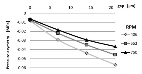
Fig. 3. Effect of gasses leaks and engine speed on compression curve asymmetry
