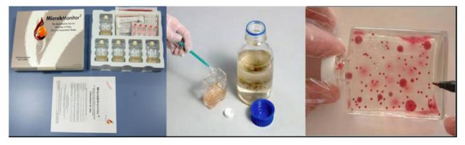
Fig. 4. Detection of microorganisms using a special kit MicrobMonitor [12]
