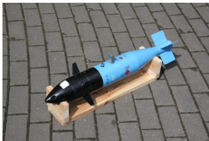
Fig. 2. LB-10M bomb with additional fins and laser seeker
