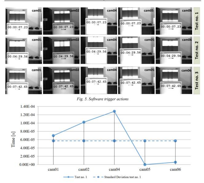
Fig. 6. The software trigger (solid line) time delay in reference to camera 5 with calculated standard deviation (dashed line)
