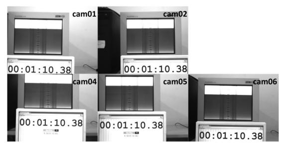
Fig. 4. External hardware trigger images assembly from five cameras
