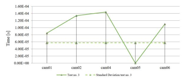
Fig. 8. The software trigger (solid line) time delay in reference to camera 5 with calculated standard deviation (dashed line)
