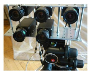
*Fig. 2. The pentadruple GigE camera array – front view*
