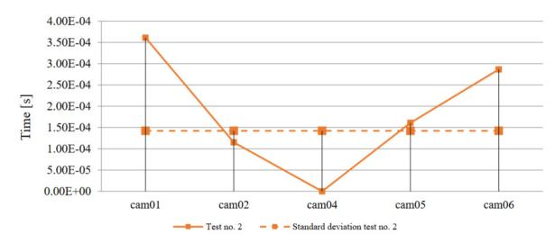
Fig. 7. The software trigger (solid line) time delay in reference to camera 4 with calculated standard deviation (dashed line)
