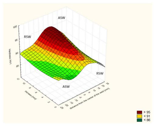
Fig. 4. Hardness distribution in joint welded by tool with conical pin, ASW – Advancing Side of the Weld, RSW – Retreating Side of the Weld
