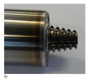
Fig. 2. View of tools used for joining by FSW: a) with cylindrical pin, b) with conical pin
