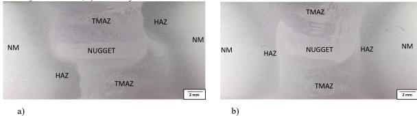
Fig. 3. Macrostructures of FSW welded joints: a) by cylindrical tool, b) by conical tool
