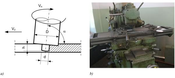
Fig. 1. The diagram of FSW (a) and view of stand used in research (b)
