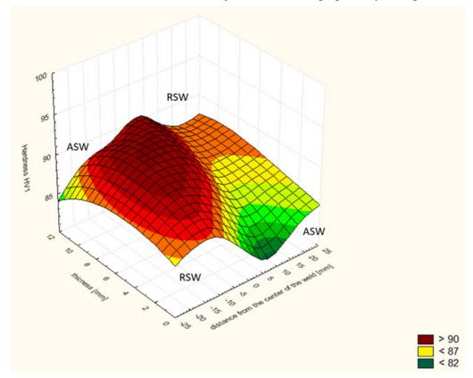
Fig. 3. Hardness distribution in joint welded by tool with cylindrical pin, ASW – Advancing Side of the Weld, RSW – Retreating Side of the Weld
