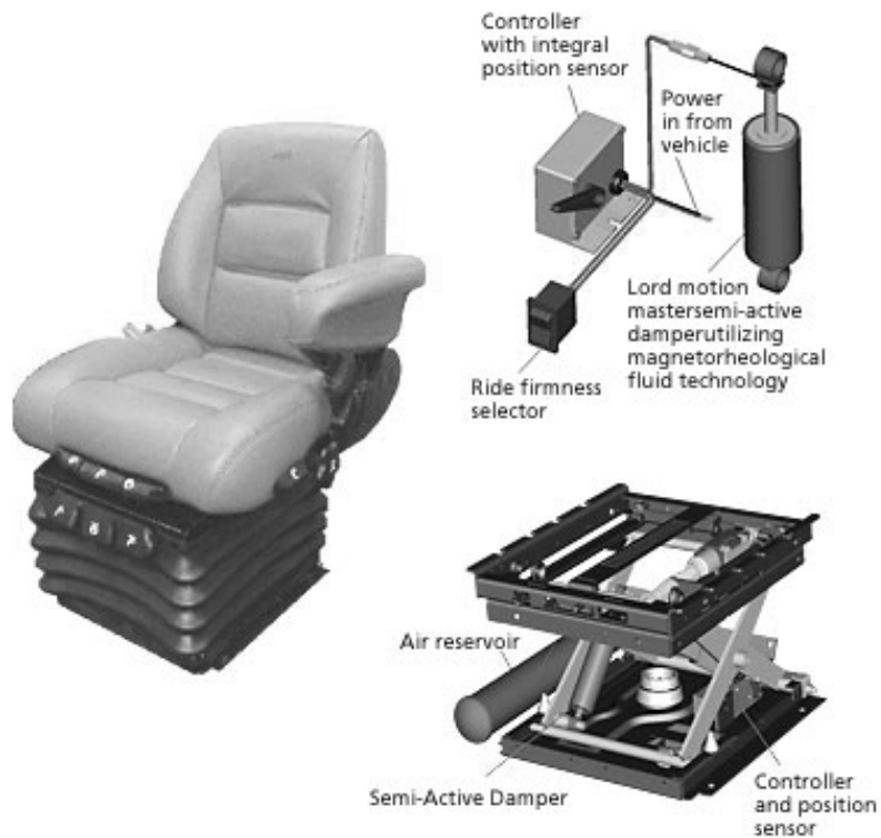
Fig. 8. Driver's seat with the vibration damping system based on MR fluid [24]
