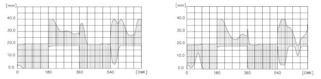
Fig. 9. Oil film height on the TR2 piston skirt for 850 rev/min (left) and 5000 rev/min (right)
