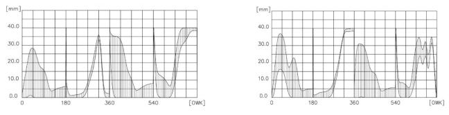
Fig. 8. Oil film height on the reference piston skirt for 850 rev/min (left) and 5000 rev / min (right)
