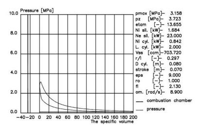
Fig. 4. Indicator diagram – idling speed
