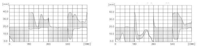
Fig. 10. Oil film height on the TR5 piston skirt for 850 rev/min (left) and 5000 rev/min (right)
