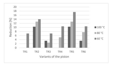
Fig. 6. The percentage reduction friction losses for all variants of the pistons to the crankshaft speed of 850 rev/min and lubricating oil temperature of 100, 80, 60°C
