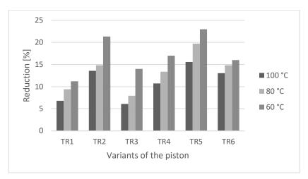
Fig. 7. The percentage reduction friction losses for all variants of the pistons to the crankshaft speed of 5000 rev/min and lubricating oil temperature of 100, 80, 60°C
