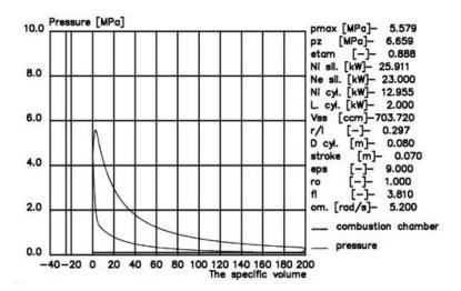
Fig. 5. Indicator diagram – full power speed
