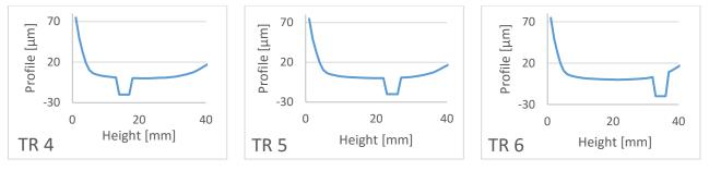
Fig. 2. TR4, TR5, TR6 variants of the piston bearing surface profile
