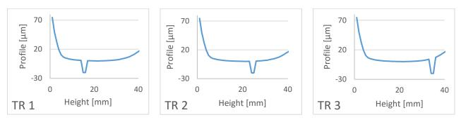
Fig. 1. TR1, TR2, TR3 variants of the piston bearing surface profile
