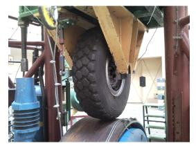
Fig. 4. Example of full scale brake test set-up
