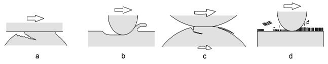
Fig. 1. Selected wear mechanisms (a – adhesive wear, b – abrasive wear, c – fatigue wear, d – corrosion wear) [5]
