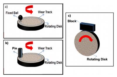
Fig. 2. Most common tribometer configurations [4]
