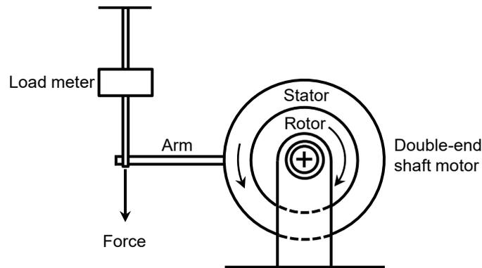
Fig. 1. Motoring friction measurement principle
