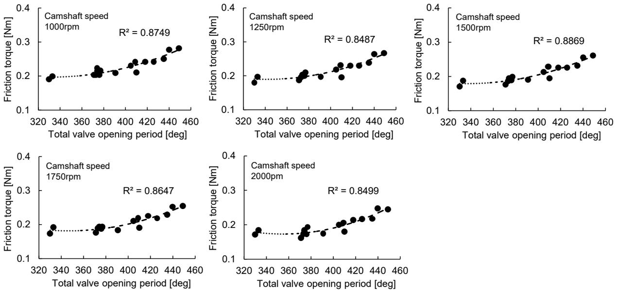
Fig. 5. Friction torque vs. total valve opening period
