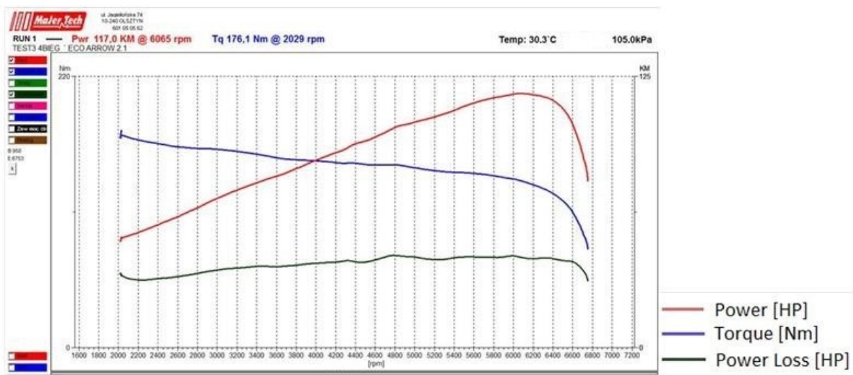
Fig. 3. Characteristics for the analysed engine. Values on the vertical axes divided by 100. Source: own studies
