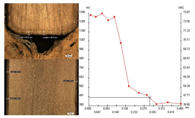
Fig. 3. Microstructure of nitrided piston ring 1-24, x100 (on the left side) and hardness distribution HV0.1 from surface to core (on the right side)
