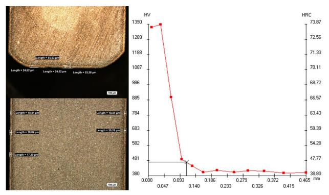
Fig. 1. Microstructure of nitrided piston ring 1-2, x100 (on the left side) and hardness distribution HV0.1 from surface to core (on the right side)
