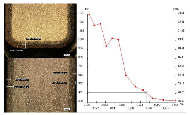
Fig. 4. Microstructure of nitrided piston ring 1-32, x100 (on the left side) and hardness distribution HV0.1 from surface to core (on the right side)
