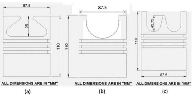
Fig. 2. Examples of studied combustion chambers [2]
