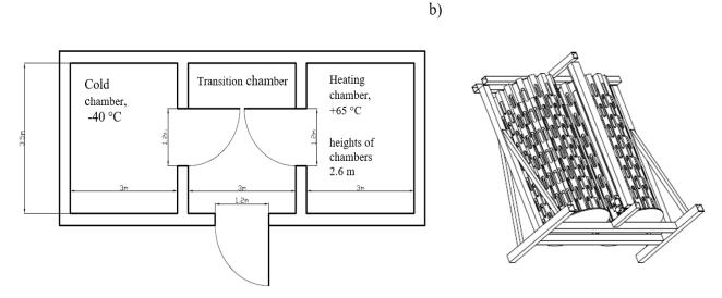
Fig. 2. Bench scheme: a) climatic chamber, b) a set of simulation tanks
