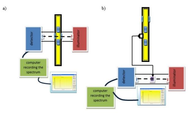
Fig. 3. Diagram of the bench for testing the ageing degree and rate of bio-components during storage: a) system of direct removal of the spectrum of the bio-component in the simulation tank, b) system of sampling and measurement in the cuvette
