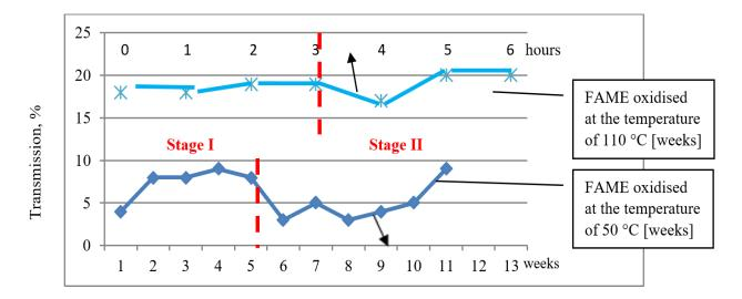
*Fig. 5.* Comparison of changes in the intensity of the 890 cm<sup>-1</sup> band derived from peroxides during the FAME sample storage under different conditions
