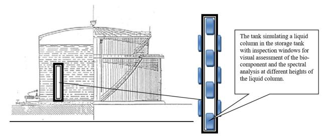
Fig. 1. Schematic diagram of the bench for testing the ageing degree and rate of bio-components during storage in the storage depots
