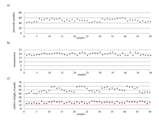
Fig. 4. Distribution of the FAME test results of: a) peroxide number, b) peak height for the wavenumber of 890 cm<sup>-1</sup> (infrared spectroscopy method), c) height of the peaks C18:1 and C18:2 (gas chromatography)
