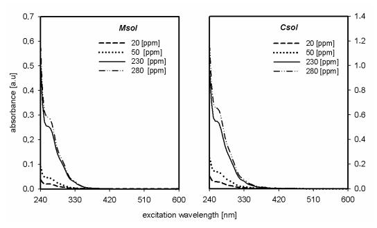
Fig. 1. Absorption spectra of oil in n-hexane for Marinol (Msol) and Cyliten (Csol) for various oil concentrations
