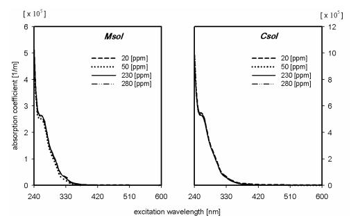
Fig. 2. Absorption coefficient of oil in n-hexane for Marinol (Msol), Cyliten (Csol) for various oil concentrations (derived using formula (2) based on the data depicted in Fig. 1)
