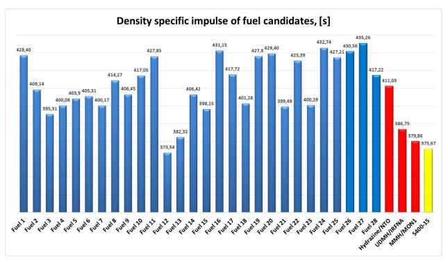
Fig. 4. The calculated density impulse of the fuel compositions based on amines, alcohols and some hydrocarbons
