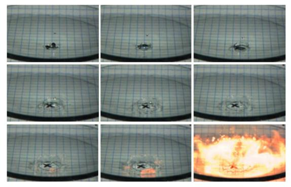
Fig. 3. The droplet test performed on energetically promoted fuel with 98% hydrogen peroxide, IDT=3.4 ms (IoA)
