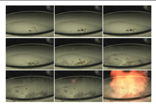
Fig. 2. The droplet test performed on catalytically promoted fuel with 98% hydrogen peroxide – the IDT=16 ms (IoA)
