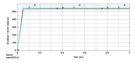
*Fig. 8. Time-velocity graph for fragments originating from opposite end – top layer*
