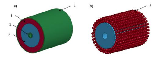
Fig. 2. Numerical model of the cylindrical fragmentation warhead a) entire model b) fragmentation liner, 1 - fragmentation liner, 2 - inner case (optional), 3 - explosive charge, 4 - outer case, 5 - steel balls
