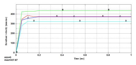
Fig. 7. Time-velocity graph for fragments originating from detonation point – top layer
