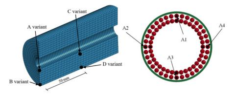
*Fig. 3. Prepared variants of the detonation point location (detonation point identified with a dot)*
