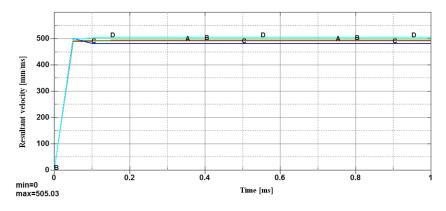
Fig. 12. Time-velocity graph for fragments originating from detonation point – top layer
