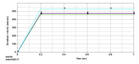
Fig. 14. Time-velocity graph for fragments originating from right end - top layer
