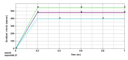
*Fig. 13. Time-velocity graph for fragments originating from left end – top layer*
