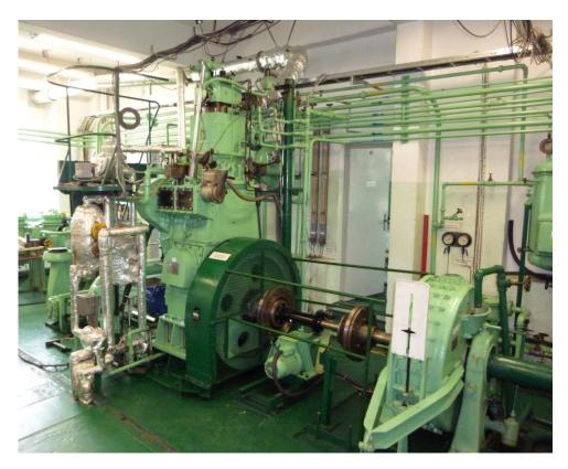
Fig. 1. Test stand with engine L-22 and water brake
