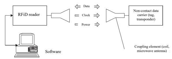
Fig. 2. The general structure of RFiD system (source [1])
