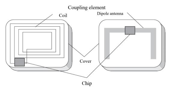
Fig. 3. The typical structure of RFiD tag (source [1])
