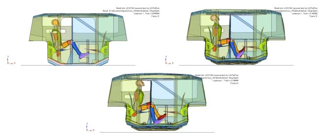
Fig. 10. Hull deformation and dummy behaviour for subsequent moments of time during detonation of 10 kg of TNT
