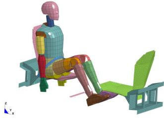
Fig. 6. Dummy positioning
