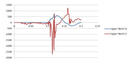
Fig. 11. Axial and transverse force in upper neck [N] during detonation of 10 kg of TNT
