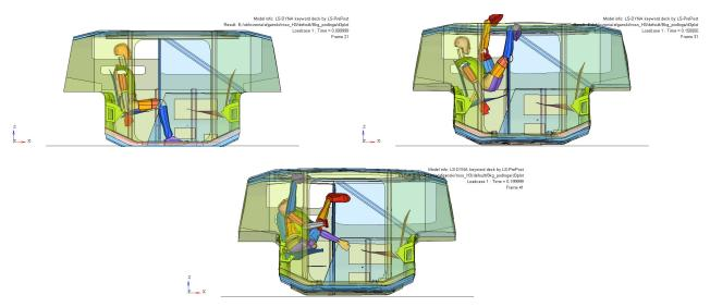
Fig. 13. Hull deformation and dummy behaviour for subsequent moments of time during detonation of 8 kg of TNT without footrest
