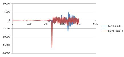
Fig. 9. Axial force in tibias [N] during detonation of 8 kg of TNT
