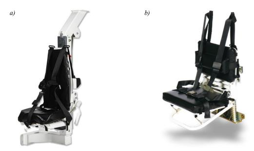
Fig. 3. Seat systems reducing overloads designed by Allen Vanguard: a) roof-mounted seat b) side-mounted seat [6]
