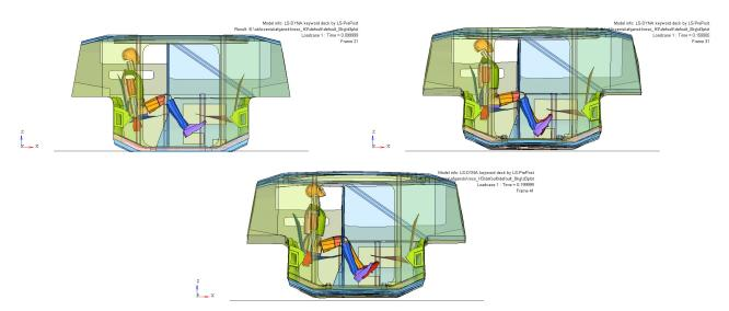
Fig. 7. Hull deformation and dummy behaviour for subsequent moments of time during detonation of 8 kg of TNT
