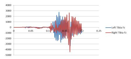
Fig. 12. Axial force in tibias [N] during detonation of 10 kg of TNT
