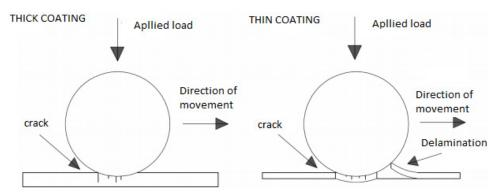
Fig. 1. Cracking of a coating in dependence of its thickness
