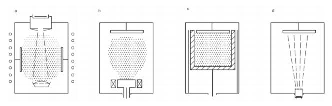
a - reactive vapourising activated by thermo-ion arch, b - vapourisation by an electric arch with an electromagnetic localization of kathode, c - direct deposition in kathode, d - straight deposition from ion clusters
