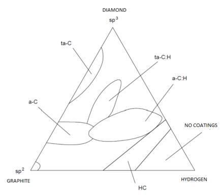
Fig. 2. Types of DLC coatings based on a chemical structure
