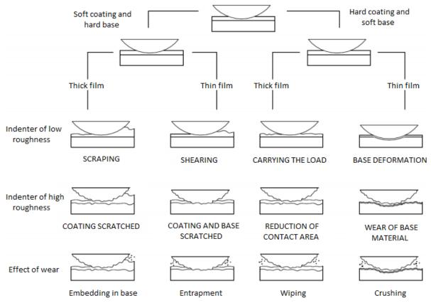
Fig. 3. Mechanism of wear for different combination of base material and coating
