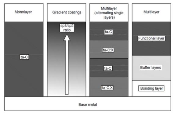
Fig. 5. Types of coatings in terms of layers number
